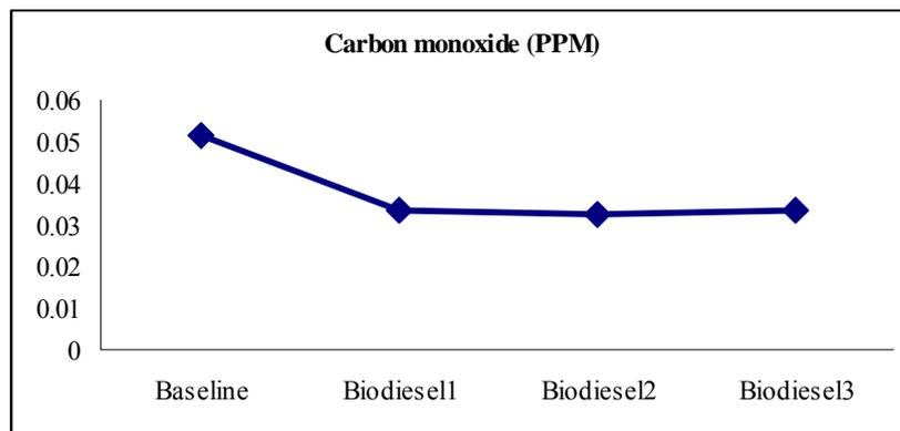
Figure 2. Carbon monoxide output baseline and with biodiesel.
