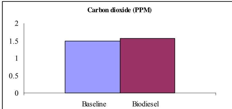
**Figure 3. Carbon dioxide output baseline and with biodiesel.**
